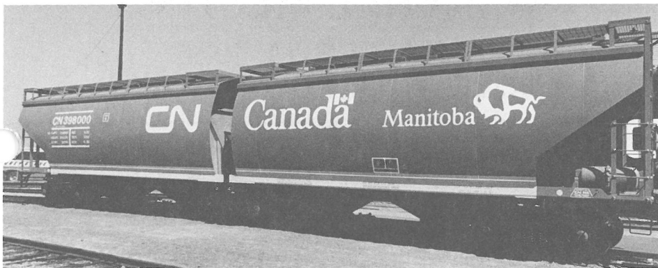
CNR's articulated grain car developed for the Churchill rail line.
